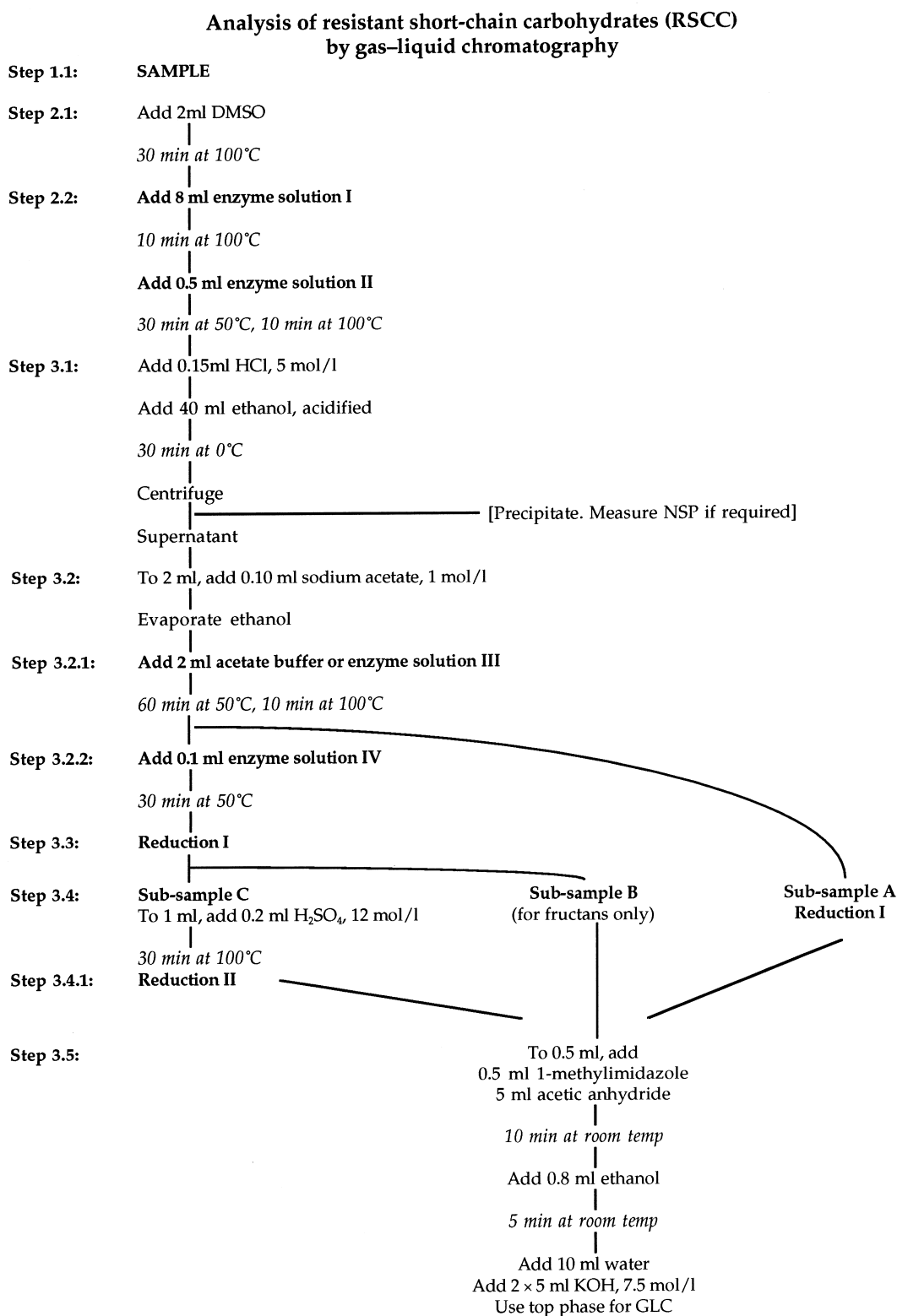
Fig. 2. A flow-chart outlining the main steps in the procedure for the analysis of RSCC by gas-liquid chromatography.
